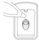
Pour rinse aid into the opening, taking care not to spill any into the drawer or on the aluminium handles.
