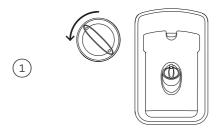
Turn the cap anticlockwise and remove.
