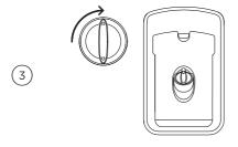
Refit the cap, turning clockwise until secure.
