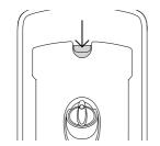
Press the latch down to open the dispenser. Check that the dispenser is empty and dry.
