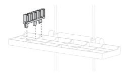
This clips onto the adjustable racks and supports knives and other utensils during the wash.
