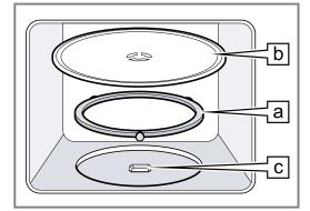
**3.** Check whether the turntable is correctly engaged. **Note:** The turntable can turn anti-clockwise or clockwise.
