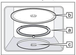
**3.** Check whether the turntable is correctly engaged. **Note:** The turntable can turn anti-clockwise or clockwise.
