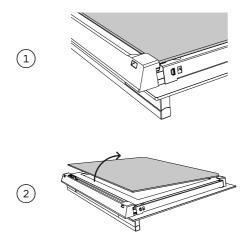
Push the glass retainer tabs in on both sides of the door. Pull the glass retainer up until the tabs relocate in the uppermost hole.
