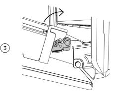
Ensure the levers are both fully locked before trying to shut the door.
