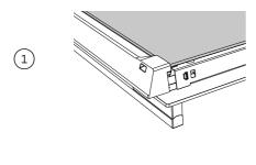
Push the glass retainer tabs in on both sides of the door again. The glass retainer can then be pulled off completely.
