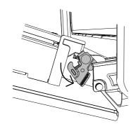
Push each locking lever down fully to release the door from the hinge.
