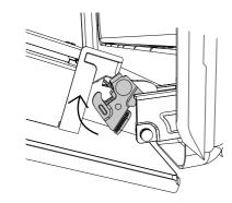
Ensure the door is firmly in place on the hinges. Open the door fully again and push each locking lever up to lock the door onto the hinge.
