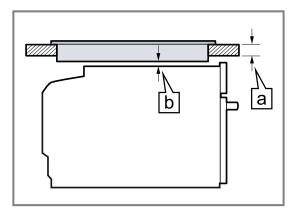
The minimum worktop thickness a is determined by the required minimum clearance b.
