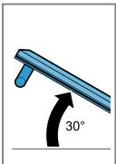
Do not close the appliance door fully. The hinges could become bent and the enamel could be damaged.
