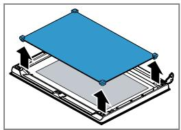
The intermediate panel is not secured using retaining pins but rather using rubber mounts.
