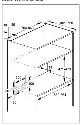
Ensure that the intermediate floor has a gap to the installation wall in order to ventilate the appliance.
