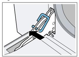
The locking pins must be fully inserted into the holes in the hinges.
