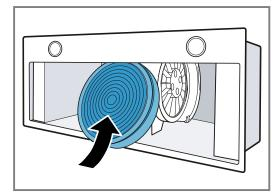
2. Guide the odour filter around the motor.
