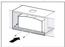
If the screws are not accessible from the exterior, the screws can also be fitted from the interior.
