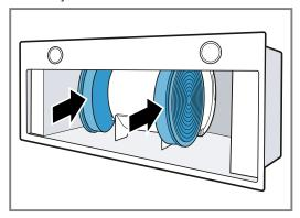
4. Install the grease filters.
