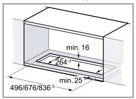
2. Make the cut-out for the exhaust air pipe either above the fitted unit or behind the fitted unit.
