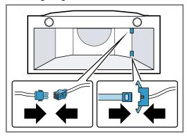
The plug can only be inserted into one position. Ensure that the connector has engaged correctly.
