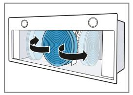
**3.** Carefully slide the odour filter into the holder.
