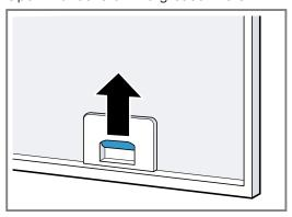
**3.** Remove the grease filters from the holders.
