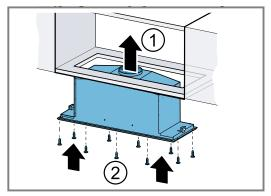
2. Tighten the fastening screws.
