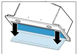
3. Undo the hinge lock and remove the filter cover.
