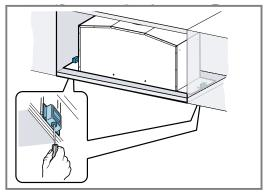
**3.** Attach the frame and screw it to the appliance from below.
