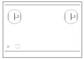
If you select settings for a different cooking zone on the same side of the cooking surface, the booster function is deactivated. The power level 9.0 is set automatically. If the function is activated in the centre of the cooking surface, you can implement the settings for other cookware on the right- and left-hand sides of the hob.
