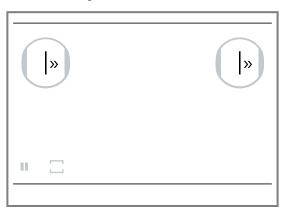
If the function is activated and you select a second cooking zone on the same side of the cooking surface, the appliance deactivates the function. The appliance automatically sets power level 9.0.
