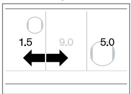
The power level of the combined area is the same as the power level of the area being expanded.
