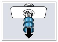
4. Press the locking catches 1 together and lift the coarse filter out ②.
