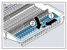
2. To fold down the front prongs, push the lever forwards and fold down the prongs ①.
