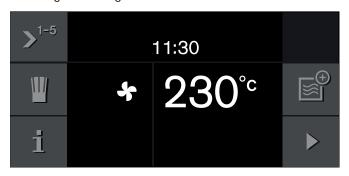
Depending on the operating mode that is selected, the right-hand control panel displays the symbol for microwave or the symbol for oven. You can use this to add the relevant other operating mode.
