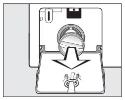
' Remove the drain filter completely.
