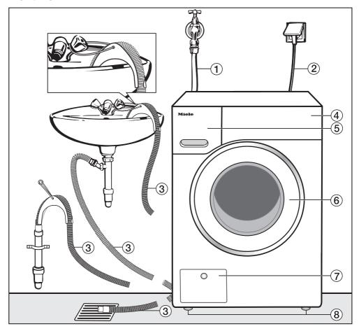
Inlet hose (tested to withstand pressures up to 7000 kPa)
