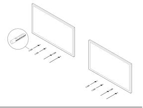
Place the bracket on the wall and loosely tighten the wall screws to secure the bracket. Check with a level and then tighten the screws.
