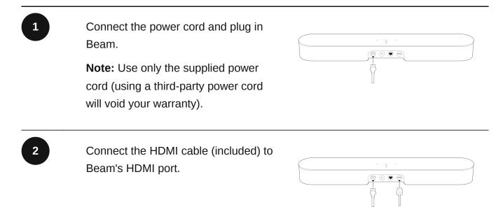
If your TV has an HDMI ARC (or eARC) port, connect the HDMI cable to it.
