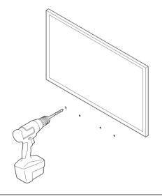
Insert and secure the wall anchors (don't use the anchors if drilling into wood).
