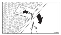
■ If the grease filter has inadvertently been refitted upside down, insert a small screwdriver blade into the slit to disengage the clip.
