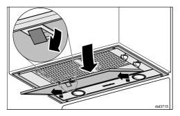
■ To take out the grease filter, release the locking clip on the filter, lower the filter approx. 45°, unhook it at the back and remove it.
