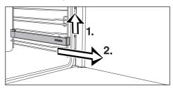
■ Remove the FlexiClip telescopic runner by raising it at the front (1.) and then pulling it forwards along the rail of the shelf level and out (2.).
