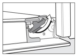
Release the locking clamps by turning them as far as they will go. The oven can be damaged if you remove the door incorrectly.
