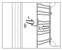
Pull the shelf runners out of the holder (1) at the front of the oven and then pull them out of the oven (2).
