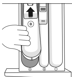
Replacing the liquid detergent compartment
