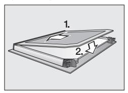
■ Push the inner pane with the matte printed side facing downwards into the plastic strip and place it between the retainers.
