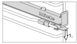
■ Push down on the tab at the front of the FlexiClip telescopic runner (1.).
