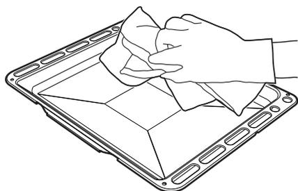
In addition to the oven cavity, the accessories (racks, trays etc.) that were used during the steam or humidification function must also be dried since the moisture on them may corrode the walls of the oven cavity and subsequently damage them.
