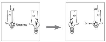
7.Refit the bracket fitting the bottom hinge pin. Replace both adjustable feet.
