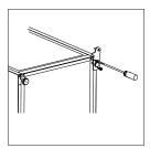
6. Unscrew and remove the bottom hinge pin with flat screw drivers, turn the bracket over and replace the pin.
