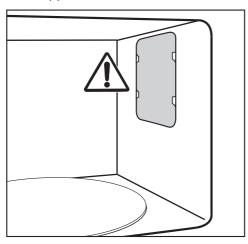
Do not remove the cover of the microwave outlet inside the oven, nor the film covering the inside of the door.
