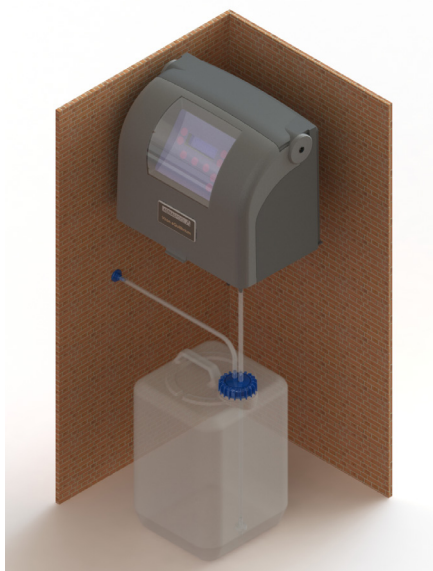
Figure 6. Acid Container Installed
