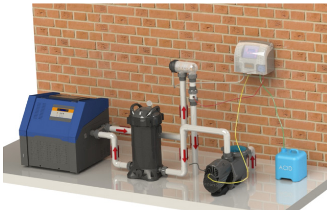
Figure 2. Equipment Configuration, Acid Dosing
