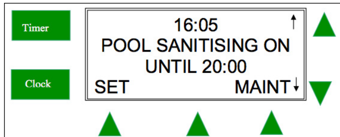
Figure 11. Chlorinator screen - SET button
