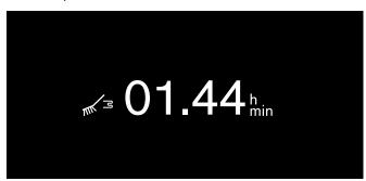
11 After 1 hour 30 minutes, a message appears in the display. Drain the used-water tank, clean it thoroughly and insert it into the appliance. Clean the fresh-water tank thoroughly, fill it with 1.7 I water and insert it into the appliance. Press to confirm.
