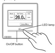
The LED lamp remains lit while the indoor unit is operating.
